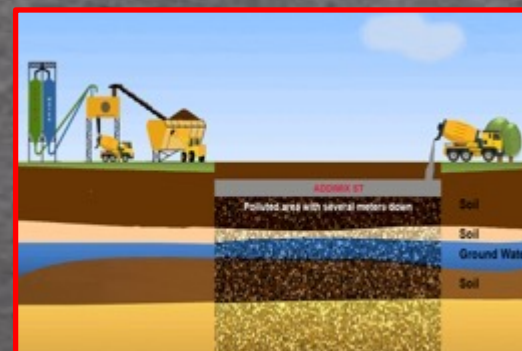
Step 3: Build a 10 cm platform to protect the ground water
