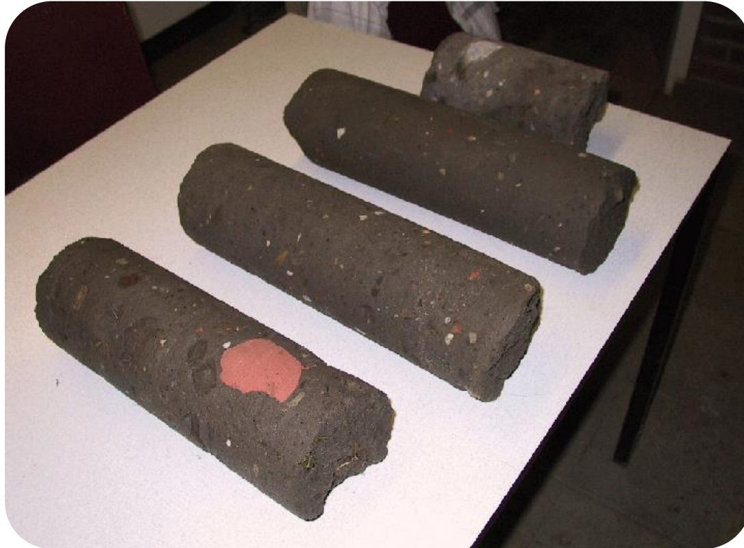
Driling cones were Sampled from the ADDIMIX base
